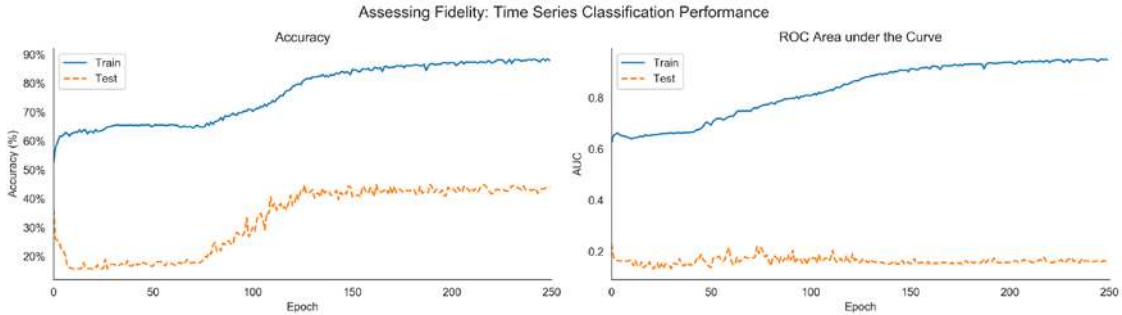
Figure 21.8: Train and test performance of the time-series classifier over 250 epochs
