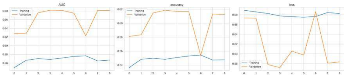
Figure 19.10: Stacked LSTM classification – cross-validation performance
